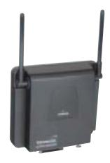
• Communicates wirelessly with personal stations through control via the main controller.
